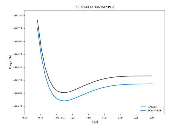
Fig. 6.20: Potential Energy Surface of the N<sub>2</sub> molecule from CASSCF(6,6) and NEVPT2 calculations (def2-SVP).
