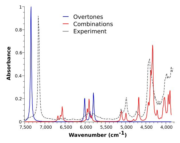
Fig. 6.48: Calculated and experimental near IR spectrum of methanol in  $CCl_4$ . The blue plot is for overtones; the red plot is for combination bands; and the grey dashed plot is the experimental spectrum. Theoretical frequencies were scaled according to literature values [442].
