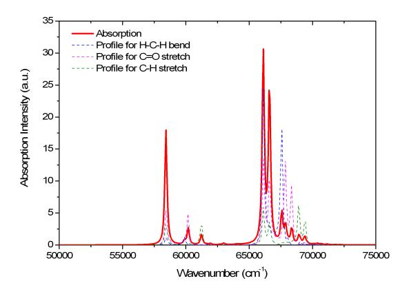
Fig. 6.44: The computed Resonance Raman excitation profiles of the three totally symmetric vibrational modes of the  $H_2CO$  molecule
