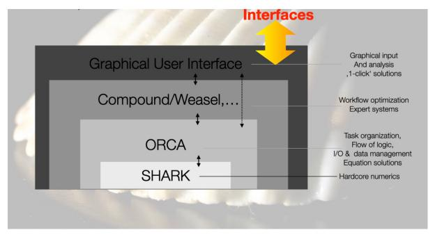
The lowest layer of the shell consists of the SHARK integral package. This is the "motor" of the program that takes care of most compute intensive tasks and essentially all parts that involve integrals over basis functions. This amounts to calculating all one- and two-electron integrals, forming Fock and Fock-like matrices and performing integral transformations using all kinds of basis sets and kernels. Most of the SHARK code is independent of the remaining ORCA source code infrastructure.
