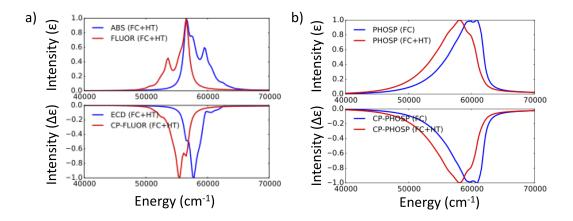
Fig. 6.70: a) Computed ABS and ECD (in blue) and Florescence and CPF (in red) under FC+HT vibronic coupling schemes b) Computed Phosphorescence and CPP under FC (in blue) and FC+HT (in red) vibronic coupling schemes
