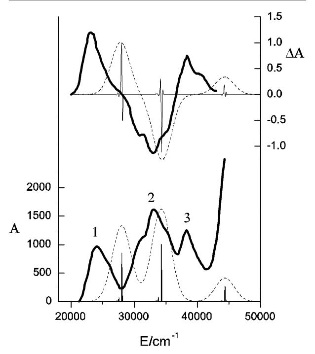
Fig. 7.41: Calculated MCD and absorption spectra of  $[Fe(CN)_{6}]^{3-}$  (dash lines) compared to experimental spectra (solid lines).
