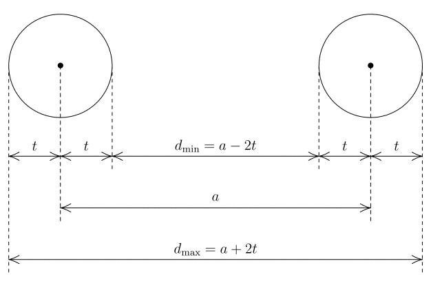
Fig. 4.1: The relation between the value t of SymThresh, the distance a of some input atom pair, and the allowed interval  $[d_{\min}, d_{\max}]$  for the distance d between the exact atom positions. This interval has the width  $d_{\max} - d_{\min} = 4t$ .
