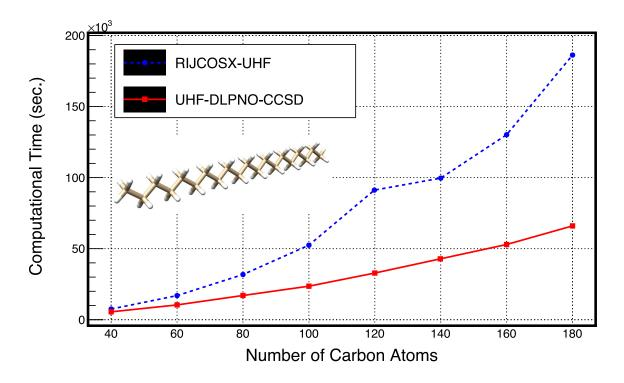
Fig. 6.7: Computational times of RIJCOSX-UHF and UHF-DLPNO-CCSD for the linear alkane chains  $(C_nH_{2n+2})$  in triplet state with def2-TZVPP basis and default frozen core settings. 4 CPU cores and 128 GB of memory were used on a single cluster node.
