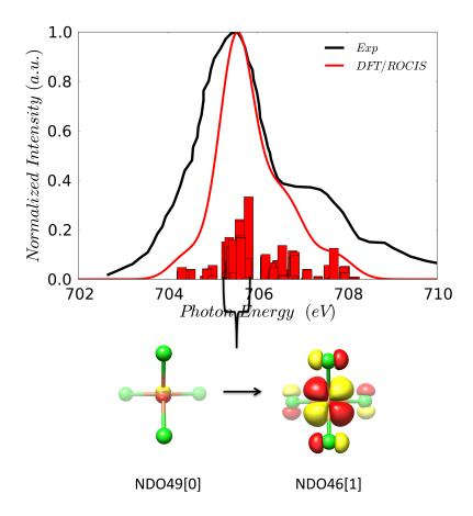
Fig. 7.33: DFT/ROCIS calculated L3 XAS spectrum of  $[Fe(Cl)_4]^{2-}$  together with NDO analysis for state 14. Constant broadening 0.5 eV and isovalue for the orbital plots 0.03 a.u. is used throughout
