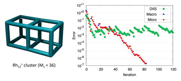
Fig. 6.10: TRAH-SCF gradient norm of a PBE/def2-TZVP calculation for a  $\mathrm{Rh}_{12}^+$  cluster in high-spin configuration ( $\mathrm{M}_\mathrm{s}=36$ ). The structure was taken from Ref. [362].
