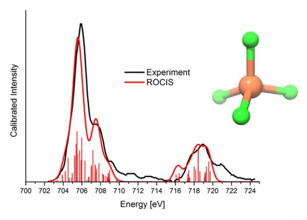
Fig. 7.31: Comparison of the experimentally observed (black) and calculated ROCIS (red) Fe L-edge of  $[FeCl_4]^{2-}$ . The red bars highlight the contribution of individual states to the total spectrum. The calculation was performed using the TZVP basis set.
