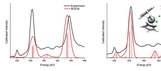
Fig. 7.32: Comparison of the experimentally observed (black) and calculated (red) Ti L-edge of  $[Cp_2TiCl_2]$ . The red bars highlight the contribution of the individual states to the total spectrum. The pure ROCIS method (left) predicts a wrong  $L_3$ - $L_2$  intensity ratio and strongly overestimates the splitting of the satellite features to the main bands. Better results are obtained with the DFT/ROCIS method (right).
