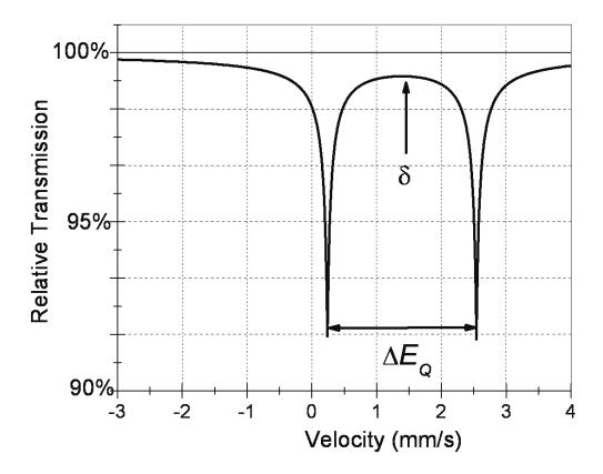
Fig. 6.56: An idealized Mössbauer spectrum showing both the isomer shift,  $\delta$ , and the quadrupole splitting,  $\Delta E_{\rm Q}$ .
