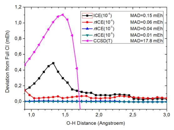
Fig. 7.15: Non-parallelity error of ICE-CI for the  $H_2O$  molecule in the SV basis. Shown is the deviation from the full CI value as a function of O-H distance (both bonds stretched). For comparison, the CCSD(T) curve is also shown
