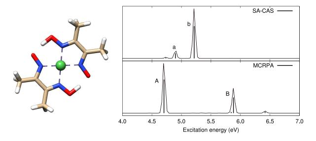
Fig. 7.35: Calculated UV/Vis spectra of Ni(dmg)<sub>2</sub>.
