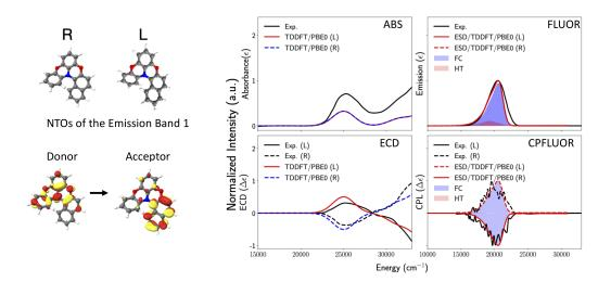
Fig. 6.71: Black Experimental vs Calculated ABS, ECD, Fluorescence and CPF spectra for R- (in blue) and L- (in red) isomers of diphenylnaphthylamine under FC+HT vibronic coupling schemes of the  $\pi \to \pi^*$  transition located at 25000  $cm^{-1}$ .
