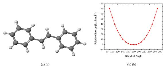
Fig. 6.33: Rotation of stilbene around the central double bond using a CASSCF(2,2) reference and correlating the reference with MR-MP2.
