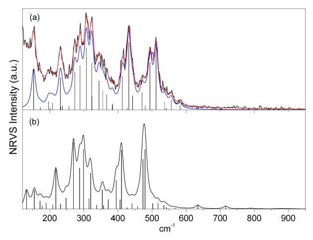
Fig. 6.50: Experimental (a, black curve), fitted (a, red) and simulated (b) NRVS spectrum of the Fe(III)-azide complex obtained at the BP86/TZVP level ( $T=20~\rm K$ ). Bar graphs represent the corresponding intensities of the individual vibrational transitions. The blue curve represents the fitted spectrum with a background line removed.
