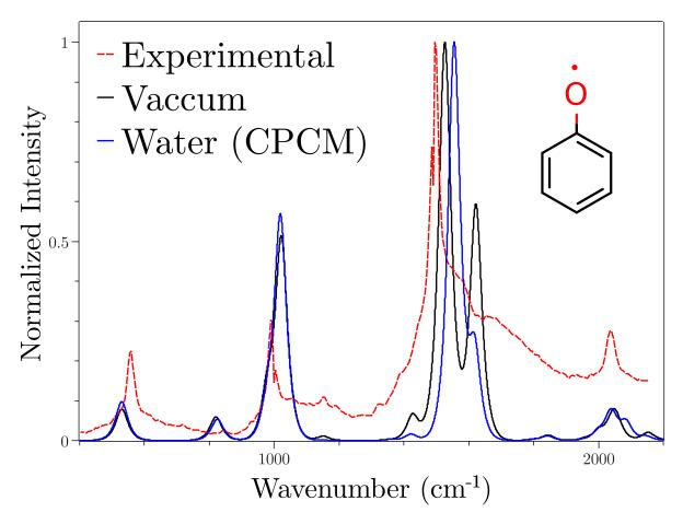
Fig. 6.67: The theoretical (solid black - vacuum and solid blue - water) and experimental (dashed red - water) resonant Raman spectrum for the phenoxyl radical.
