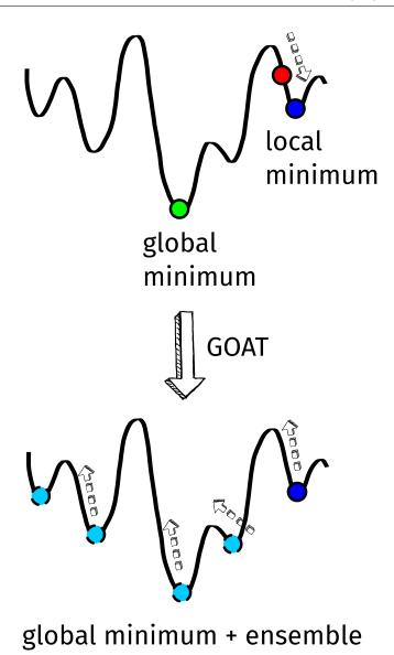
Fig. 6.24: A simple depiction of the difference between a regular geometry optimization (above), and the GOAT global optimizer (below). By using the latter, one finds not only one local minimum but the global one and the
