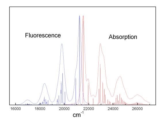
Fig. 7.45: Absorption and fluorescence spectra generated after orca\_asa run on the file example003.inp. Also, the high-resolution spectra corresponding to homogeneous broadening  $\Gamma=10\,\mathrm{cm}^{-1}$  are shown.
