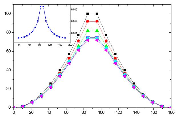
Fig. 6.1: A rigid scan along the twisting coordinate of  $C_2H_4$ . The inset shows the  $T_1$  diagnostic for the CCSD calculation.
