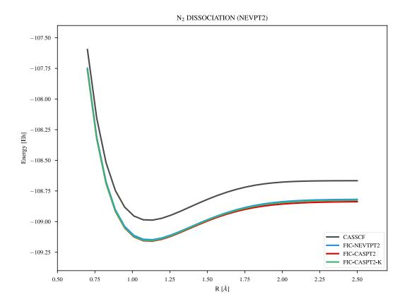
Fig. 6.21: Potential Energy Surface of the N<sub>2</sub> molecule from CASSCF(6,6) and CASPT2 calculations (def2-SVP).
