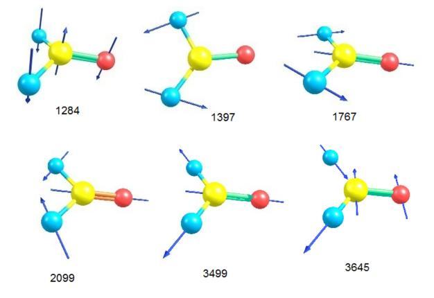
Fig. 6.52: Normal modes of  $H_2CO$  with arrows indicating magnitude and direction of nuclear motions and the associated vibrational frequencies in cm<sup>-1</sup> obtained from ORCA output file through the use of ChemCraft
