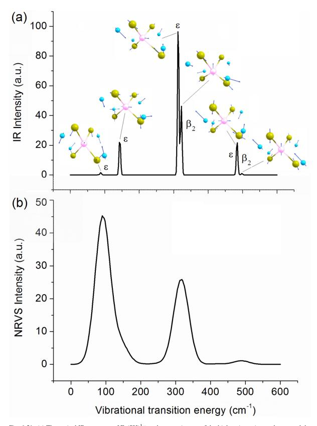
Fig. 6.51: (a) Theoretical IR spectrum of  $Fe(SH)_4^{1-}$  and arrow-pictures of the highest intensity modes around the peak maxima. (b) The corresponding NRVS scattering spectrum.
