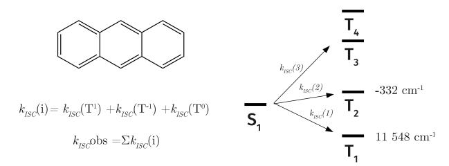
Fig. 6.66: Scheme for the calculation of the intersystem crossing in anthracene. The  $k_{ISC}(i)$  between  $S_1$  and each triplet is a sum of all transitions to the spin-sublevels and the actual observed  $k_{ISC}^{obs}$ , which consolidates these transitions. On the right, there is a diagram illustrating the distribution of excited states with  $E(S_1) - E(T_n)$  depicted on the side. Since  $T_3$  is energetically too high, intersystem crossing involving  $T_3$  can be safely neglected.
