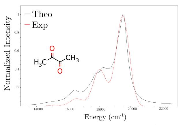
Fig. 6.65: The experimental (dashed red) and theoretical (solid black, displaced by about 2800 cm<sup>-1</sup>) phosphorescence spectra for biacetyl, in ethanol at 298 K.
