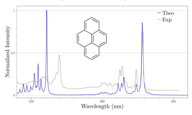
Fig. 6.61: Predicted absorption spectrum for pyrene in gas phase (solid blue) in comparison to the experiment (dashed grey) at 298 K.
